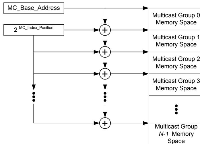
**Figure 6.xx: Segmentation of the Multicast Address Range**
