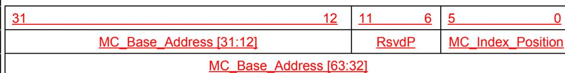
**Figure 7-xx MC Base Address Register**
