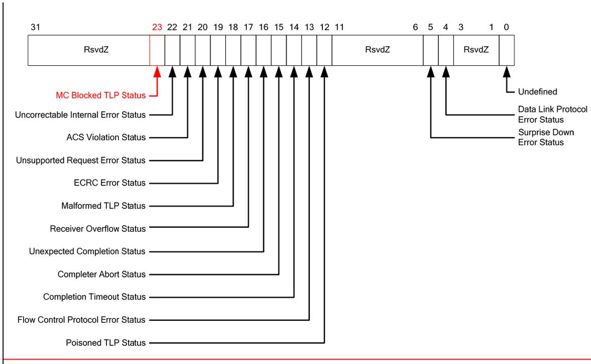
Figure 7-32 Uncorrectable Error Status Register
