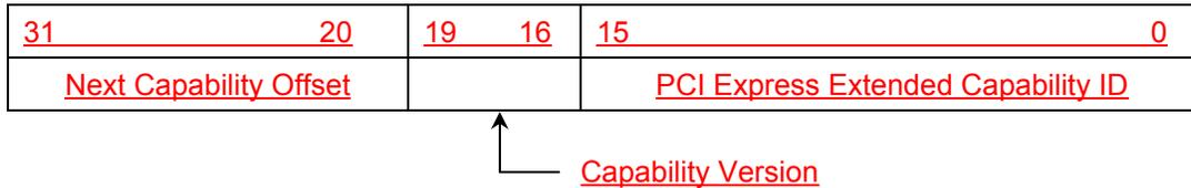
**Figure 7-xx Multicast Extended Capability Header**
