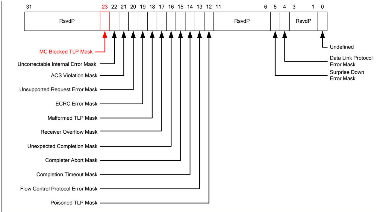
Figure 7-33: Uncorrectable Error Mask Register
