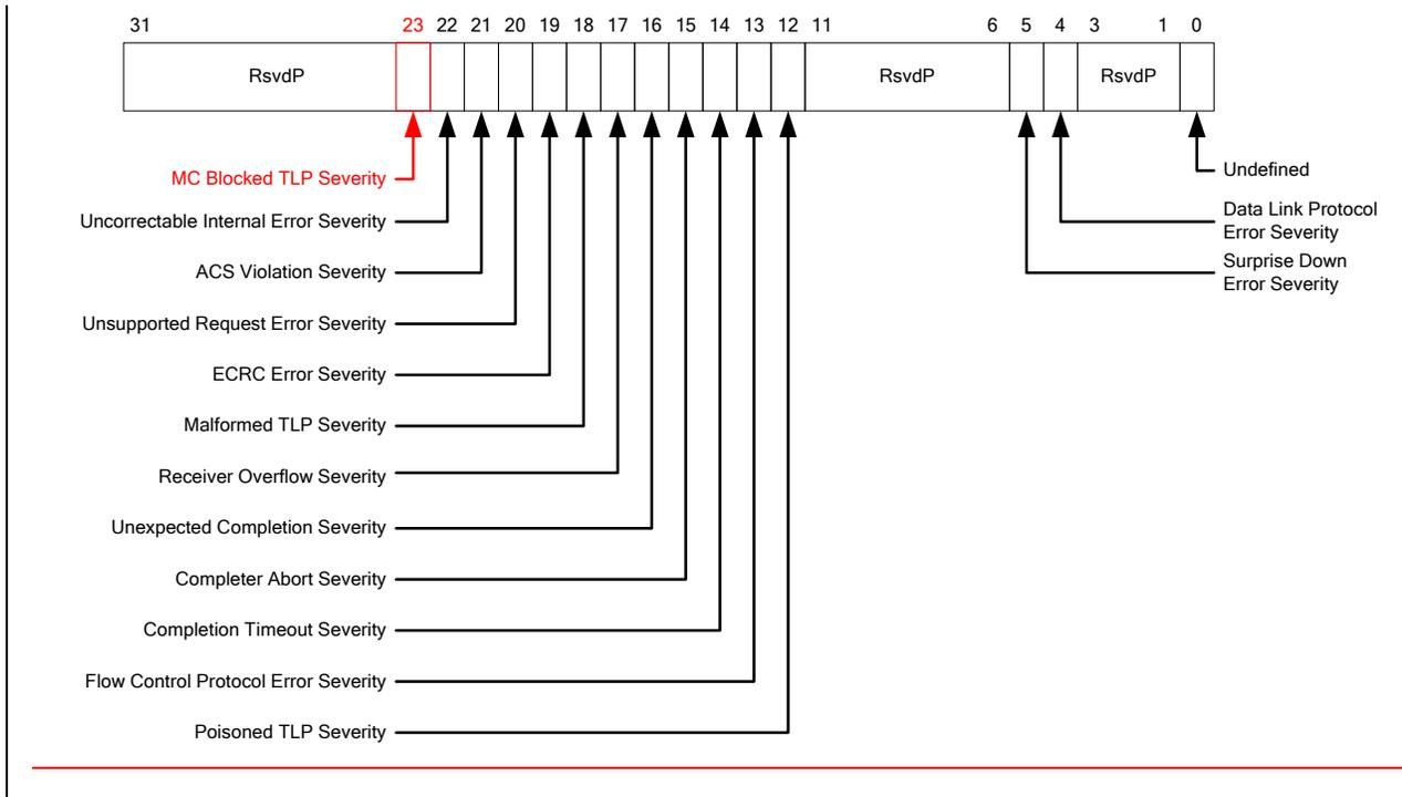
Figure 7-34: Uncorrectable Error Severity Register
