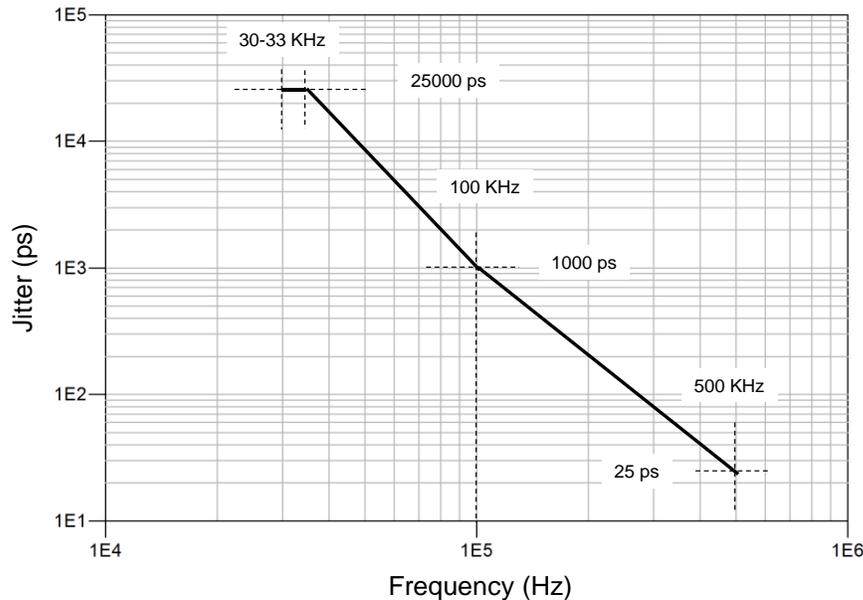
Figure 4-x1: Limits for phase jitter from the Reference Clock
