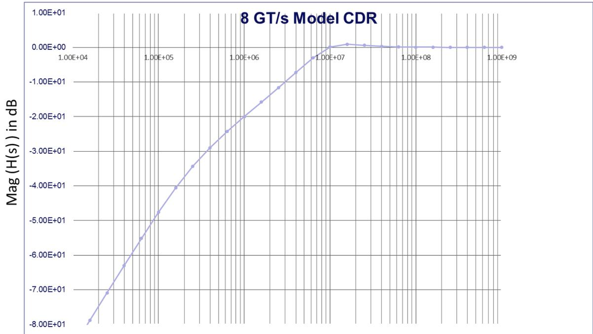
Figure 4-9x2: Informative CDR Jitter Transfer Function for the Separate Refclk With Independent SSC (SRIS) Architecture at 8.0 GT/s
